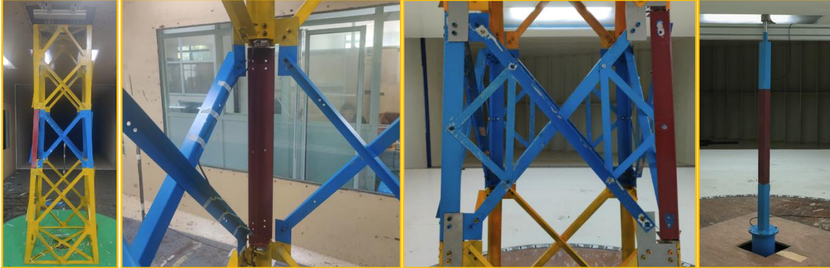
Figure 1. Models in the wind tunnel: a) the lattice structure model; b) details of testing member; c) ways of change solidity ratio; d) the single angle member model.
